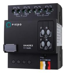
SHADE2 is a professional two curtains(shutters) controller. The curtain module can only control the curtain by AC motor. Each curtain can set running time for closing the AC power if the curtain limit switch is failed. Each channel has inching function, it allows users to control the motor in short time, such as changing the angle of shutter. Pieronet can control the curtain from iPad, iPhone local and internet.
