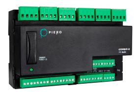
The COMBO-2 Hotel I/O module is a mix module. It has dimming function of MOSFET tube, relay, curtain control, dry contact and three LED outputs functions. The 3 indicators of the indoor door bell can be controlled by the panel universal switch. The output channel parameters can be set via PieroNet Software. After setting, the targets (curtains, lights, fans etc,) can be controlled by the panel.
