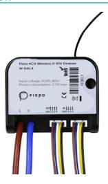
W-BAL4 PieroNet Wireless 4CH DC0-10V Dimmer. It has 4CH for 0-10V output, you can adjust the LED value by electronic ballast. And it has 4CH dry contact, can control target by switch. This module should be configured with mesh gateway.
